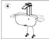
4. After the installation, turn on the water valves to check if there any leakage. Lift the tap handle up and down to turn on/off the water. Turn the handle left and right to adjust the water temperature. For the first time use, leave the water on for at least 15 seconds to clean up the pipe (as shown in diagram 4).
