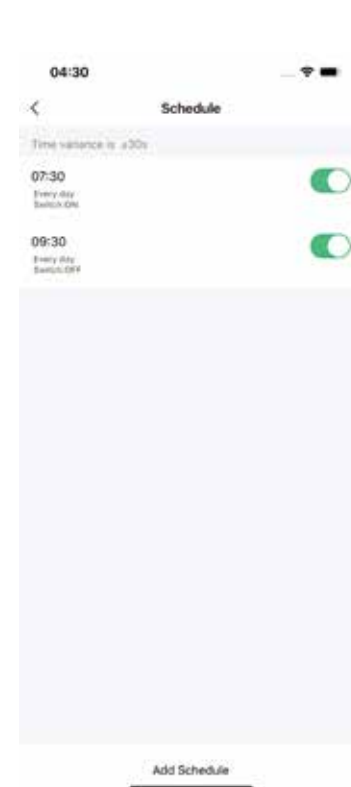
18. A schedule only supports the operation of the electric towel rack to open or close. If you need to make it automatically open and close automatically, you need to set up two schedules to realize this function.
