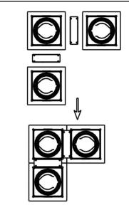
Three single units assemble with two connectors to be "L" shape triple unit.
