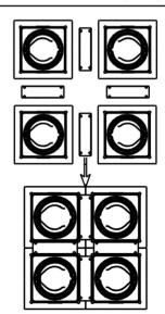
Four single units assemble with four connectors to be quadruple unit.
