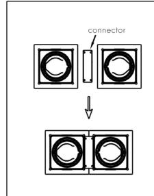
Two single units assemble with two connectors to be double unit.
