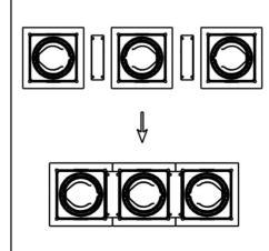
Three single units assemble with two connectors to be triple unit.
