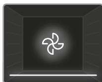
**Lower Heating and Fan Function:** The oven's thermostat and warning lights will switch on, and the lower heating element and fan will start
