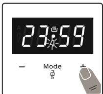
2. Select the desired time period using the **"+"** and **"-"** keys while **"K"** is flashing.
