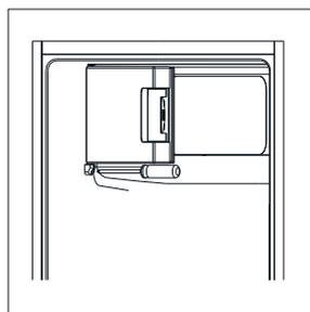
**Step 7:** Rotate freezer door and place hinge at left side and then fix the door by the holder.
