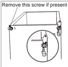
**Step 8:** Unscrew bottom hinge. Then remove the height-adjustable feet from both sides.
