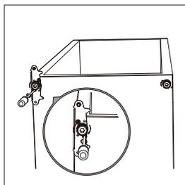
**Step 10:** Refit the bracket fitting the bottom hinge pin. Replace both height-adjustable feet.
