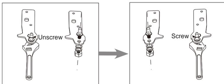
**Step 9:** Unscrew and remove the bottom hinge pin, turn the bracket over and replace it.
