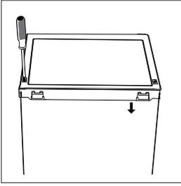
**Step 12:** Put the top cover and fix it with the two screws on the back.
