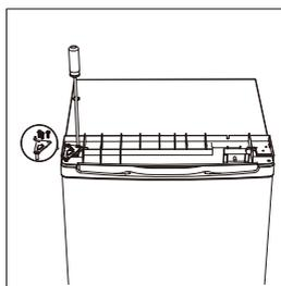
**Step 11:** Place the door back on. Ensure the door is aligned horizontally and vertically so that the seals are closed on all sides before finally tightening the top hinge.
