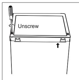
**Step 1:** Remove two screws at rear side of top cover.
