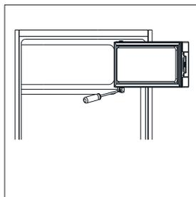
**Step 4:** Unscrew bottom hinge of freezer door and then remove door and place it on a soft pad to avoid scratches.
