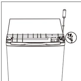
**Step 3:** Unscrew top hinge and then remove door and place it on a soft pad to avoid scratches.
