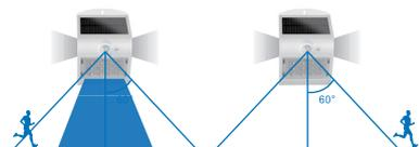
**Mode B:** Automatically turns on to full brightness (220lm) when motion is detected in the range  $\leq 6$  mtrs and then turns to weak brightness (front light off & back light on) in 10 seconds of no motion.
