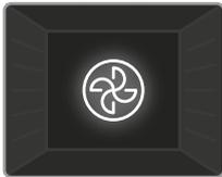
**Turbo Function:** The oven's thermostat and warning lights will switch on, and the ring heating element and fan will start operating. The turbo function evenly disperses the heat in the oven so all food on all racks will cook evenly. It is recommended that you preheat the oven for about 10 minutes.
