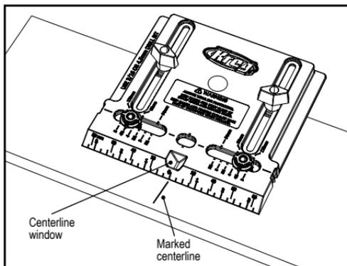
**Additional Alignment Features:** For centering a knob up to  $3\frac{1}{2}$ " [89mm] from the top or bottom edge of a door, use the inch or millimeter scales on the beveled edge of the Base.
