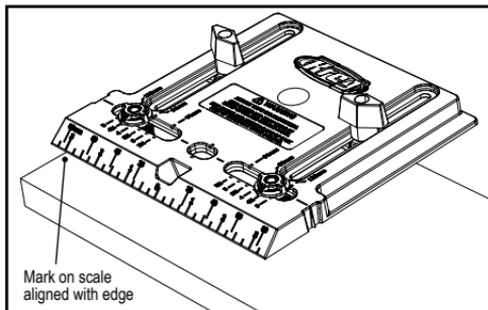
For aligning the Cabinet Hardware Jig at distances beyond the 5" [127mm] capacity of the Edge Guide, mark horizontal and vertical centerlines on your workpiece, remove the Edge Guide, and align the Jig by using the Centerline Pointers at the edges of the Base and the Centerline Window.
