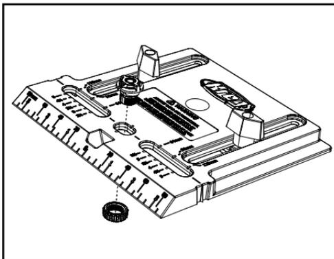
Adjust the Edge Guide to the desired distance from the edge of the workpiece on which you wish to mount the pull or knob. For dimensions in inches, align the arrows at the ends of the Edge Guide with the appropriate dimension on the inch scales along the edges of the Base. For dimensions in millimeters, align the back edge of the Edge Guide with the appropriate dimension on the millimeter scales along the inside edges of the Edge Guide adjustment slots. Tighten the T-Knobs.
