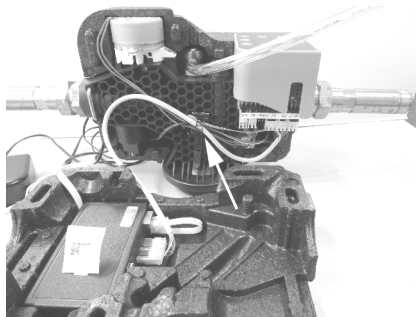
Fig. 9: Insert cable into cable tie
