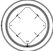
5. Press the buckle outwards, remove the aluminum substrate from the buckle, and remove the light source board.
