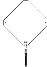
6. Take out two-cord cable (wire diameter 18-22AWG) and insert it into the plug-in terminal. Connect the external power supply for testing.
