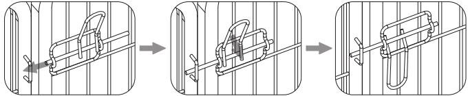
Lock the swing door by gripping the handle of the bar and pushing it into the latch.
