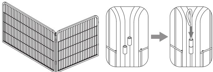
Place two units next to each other's frames. Hold the drill holes of the hinge level. Insert one of the anchoring hooks through the holes.
