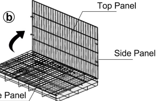
Unlatch Locking Device located on side of crate Grab any wire on the top panel and turn it like the page of a book. then garb top and side panel and pull upwards.
