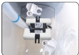
1. Remove the foam around the pump
