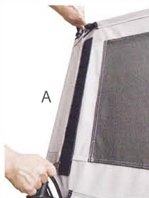
**EN** Pull hard over the metal pipe A, then stick the velcro. (see note 3)
