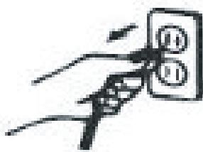
Please do not use with wet hands on the plug and while operating as this may cause an electric shock or a fire.
