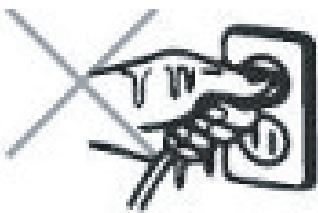
When pulling out the plug, do not pull directly on the power cord but pull out the plug as this may cause an electric short circuit and fire.
