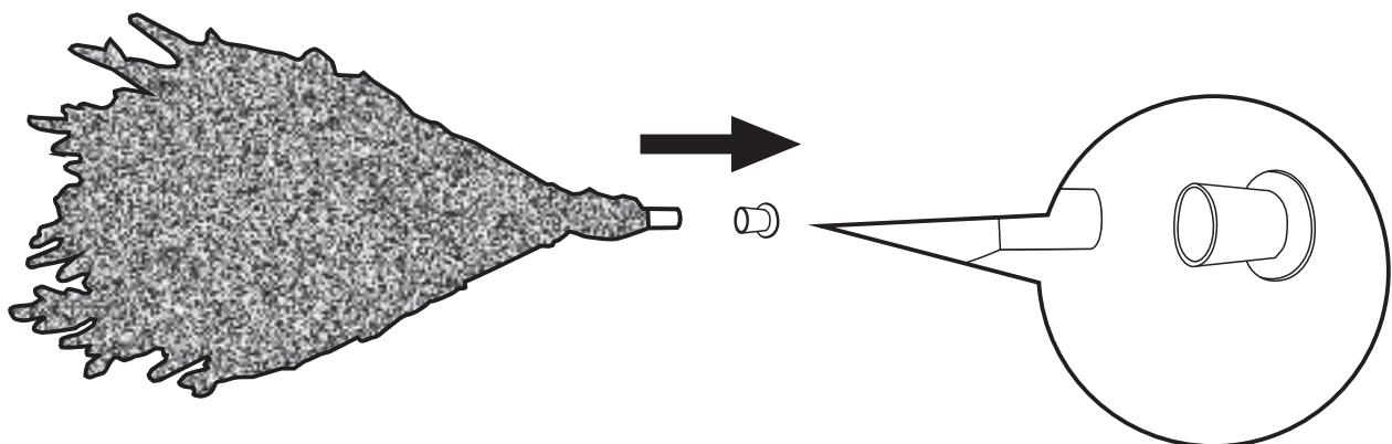
**EN\_NOTE:** Please remove the circular protector caps on the end of each pole before assembling.
