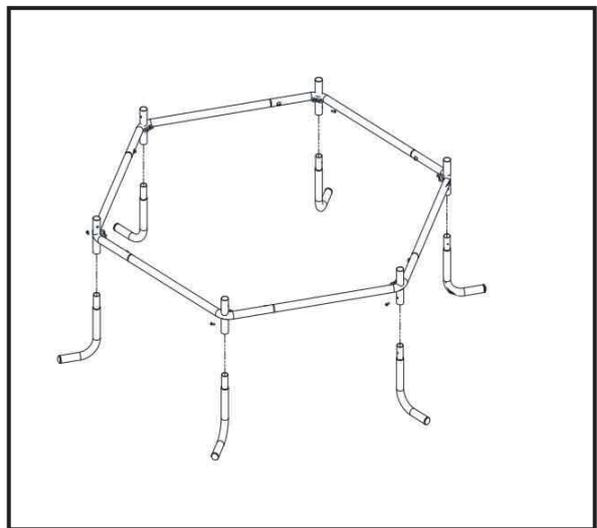
2. Install the “L” leg tube into the main rack in turn and tighten the screws by tool.
