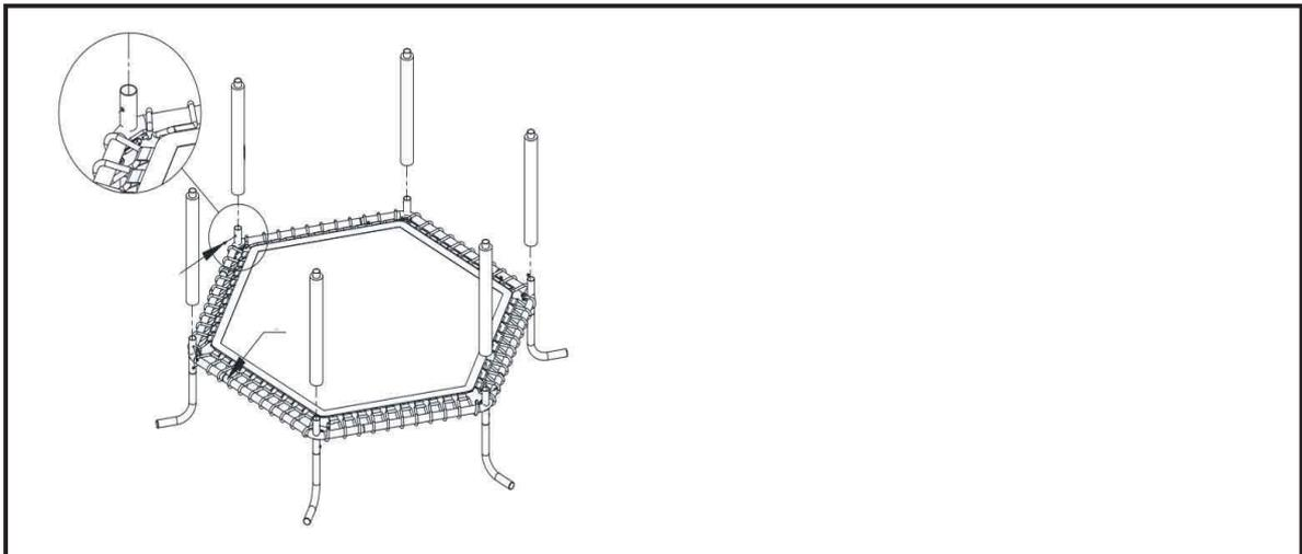
5. Secure the net from the top down to the main rack with the fastening buckle of the net on the ball head and tie the elastic band below to the pipe below.
