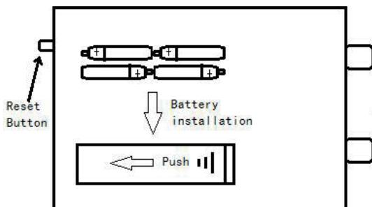
**Step1:**When door is open,open the battery compartment,and insert batteries.
