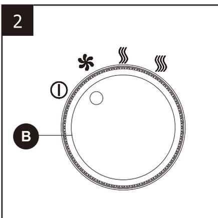
3. Set the temperature by turning the thermostat knob on the control panel (B).
