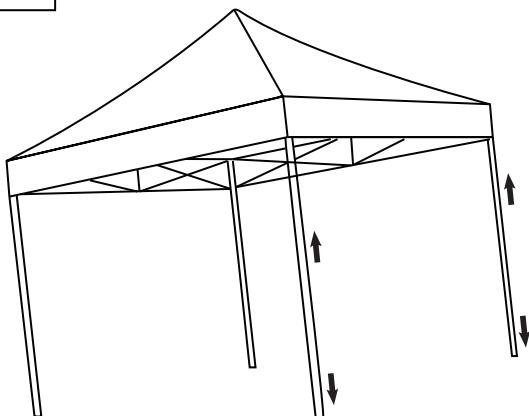
4. Lift two adjacent outer legs up and pull out the inner legs until snap locks. Repeat on all legs. Raise or level the shelter using adjustment holes found near bottom of each outer leg.
