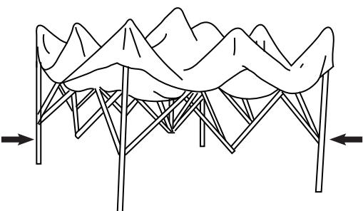
3.Grasp top of diamond on opposite sides,lift up,shake shelter a little while stepping towards partner until unit is 3/4 closed.Grasp two outer legs,push together to fully close(do not pinch fingers).Put on cover bag.
