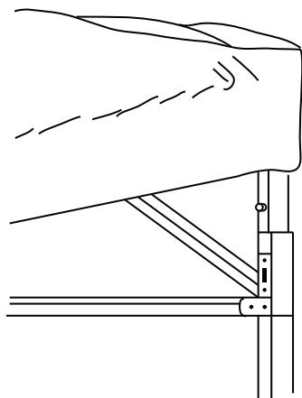
3. Engage the auto slider at each corner by pushing up with one hand while holding down top of leg with the other hand. Snap button will engage in groove. Repeat on all other legs.
