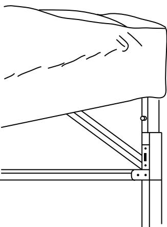
2.Release auto slider at each corner by pushing Snap-Button to release pressure on slider.Repeat on all four corners.
