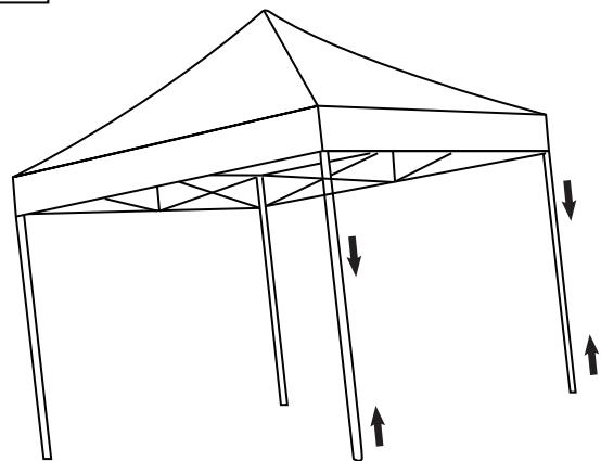
1.Lift two outer legs slightly,depress snap button,telescope inner legs up into outer legs.Repeat on opposite side.
