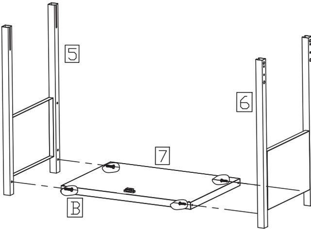
1. Assemble the LH and RH frame (5&6) to bottom shelf (7) with 4pcs M5 screws (B).
