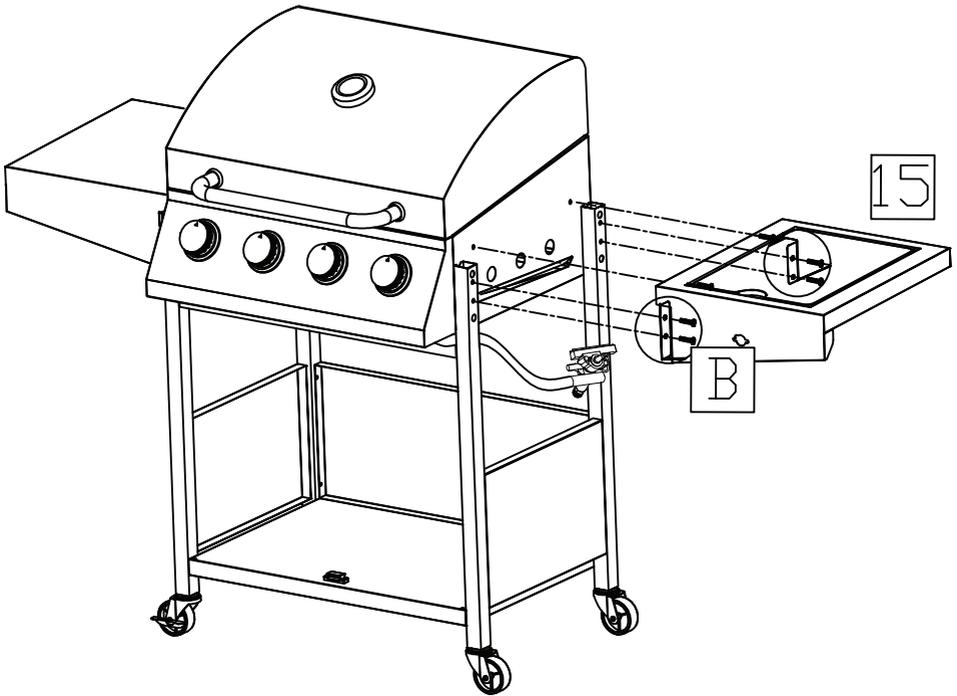
7. RH side shelf (14) is assembled to the body with 6 pcs M5 screws (B).
