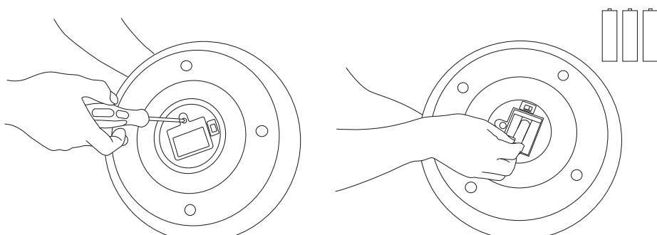
1 Unscrew the battery compartment cover with a screwdriver.
